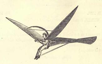
A hinged tail of an inverted trough form is attached to the rear of the frame, and may be actuated by cords attached to the feet of the aëronaut.
